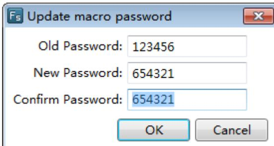
Enter the correct old password and valid new password, then clicking the button “OK” to confirm the password modification.
