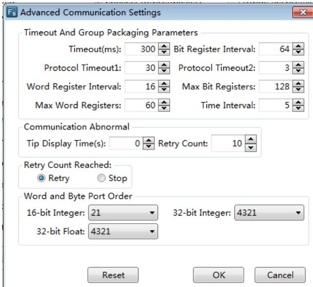
The parameters in the Advanced Communication Settings should not be modified, unless the professional guidance is given. The optional modification may result in a communication failure or unexpected events occur. You can consult the factory technical staff to modify the advanced parameters based on your needs. In most cases, the default parameters are the best and need not to be changed.
