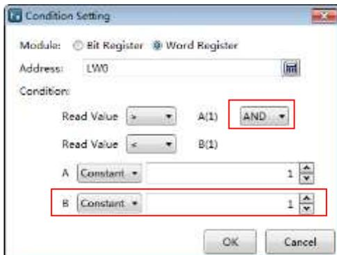
If the conditions you need is "LW0 > 100" and "LW0 < LW1", then the condition of the second is not "constant" but "variable" and the address is LW1. The setting is shown as below.
