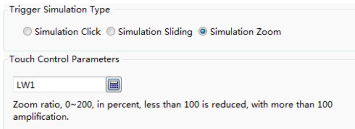
When the trigger conditions of the touch trigger component are met, the components which occupy the active area of the touch trigger component will execute the zooming action within this area, such as viewing the trend curve by zooming.
