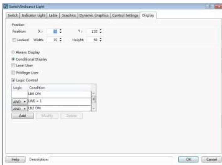
The “X” and “Y” in the Position property are used to set the x coordinate and the y coordinate of the start point of the current component in the window. The title of the “X” and “Y” is “Fixed Point” or “Position”. The title of "Fixed Point" decides a fixed point as the start point of the component. The detail is referred to: [Detailed manual/ General functions/ Drawing/ Rotation](#). The title of "Position" decides the point in the upper left corner of the component as the start point.
