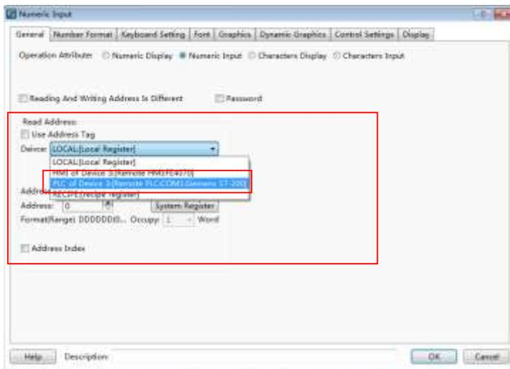
After finishing setting the "Remote PLC", the local HMI can access all the registers of the "Remote PLC" which is connected to the "Remote HMI".
