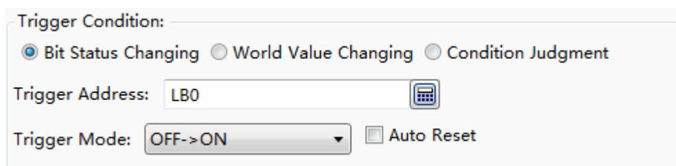
The “Trigger Condition” supports “Bit Status Changing”, “Word Value Changing” and “Condition Judgment”. The settings are referred to: [Detailed manual/Component/Timer and Data Transmission/Timer](#).
