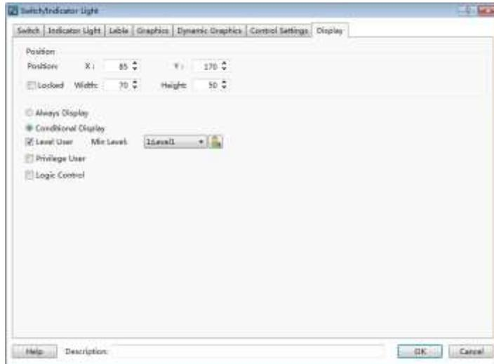
If you check this function, the component will be visible after you entering the appropriate user level password.
