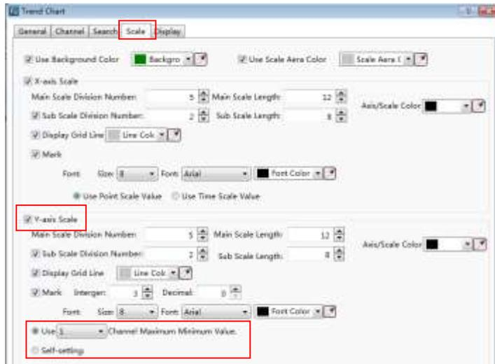
After you select the option “Use ... Channel Maximum Minimum Value”, you can specify a channel number. And the minimum and the maximum values of this channel will be used as the minimum and the maximum values of the Y axis.
