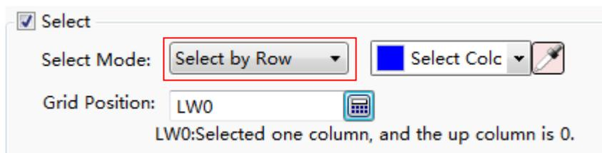
You need to give a word register to record the selected column number if the select mode is “Select by Column”. The first column number is 0.
