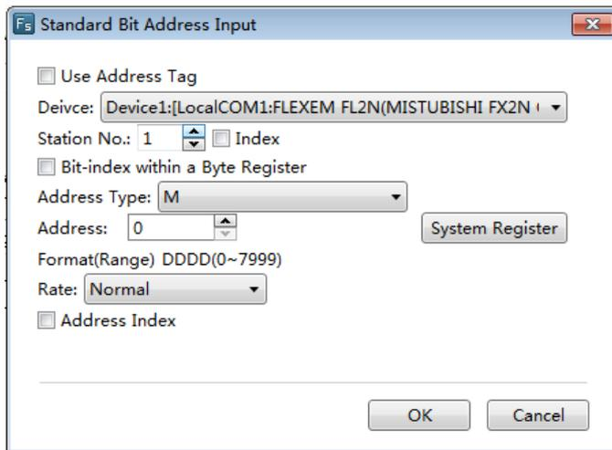
In the VEDA HCT software, the corresponding bit address symbols are given according to the various connected devices. For the Flexem FL2N series PLC, X represents the input address, Y represents the output address, M represents the middle register address, SM represents the system special bit address, and S represents the state address. As shown as below.
