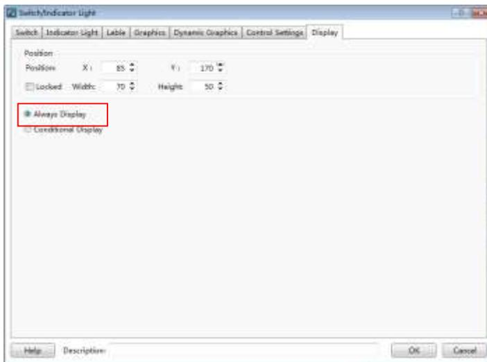
If you select the “Always Display” function, the component will always be visible when the project is running. It is the default setting.
