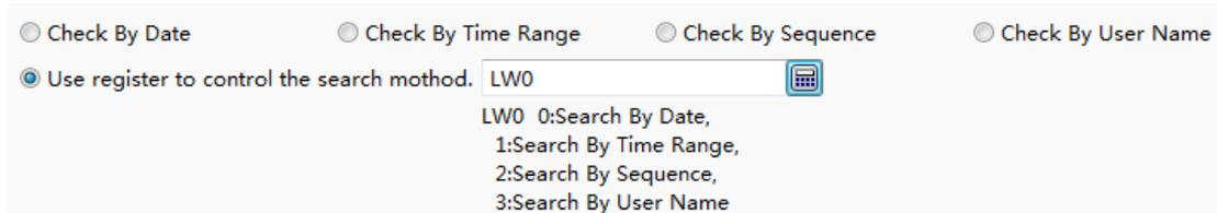
The screenshot shows a search configuration interface. At the top, there are four radio buttons: "Check By Date", "Check By Time Range", "Check By Sequence", and "Check By User Name". Below these is a checked radio button labeled "Use register to control the search method." followed by a text input field containing "LW0" and a calendar icon. Underneath the input field, there is a legend: "LW0 0:Search By Date, 1:Search By Time Range, 2:Search By Sequence, 3:Search By User Name".
