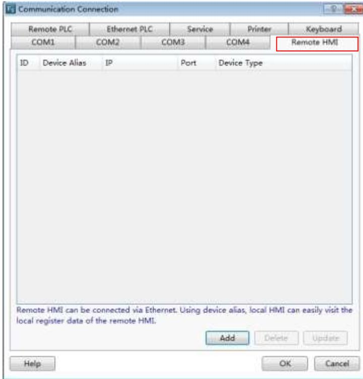
For one of the HMI device, anyone of other HMI devices in the same Ethernet network of the LAN is the Remote HMI. For example, there are two HMI: one named HMI1, another one named HMI2. These two HMI devices are connected in an Ethernet network. For HMI1 device, HMI2 is the "remote HMI" of HMI1. For HMI2 device, HMI1 is the "remote HMI" of HMI2.
