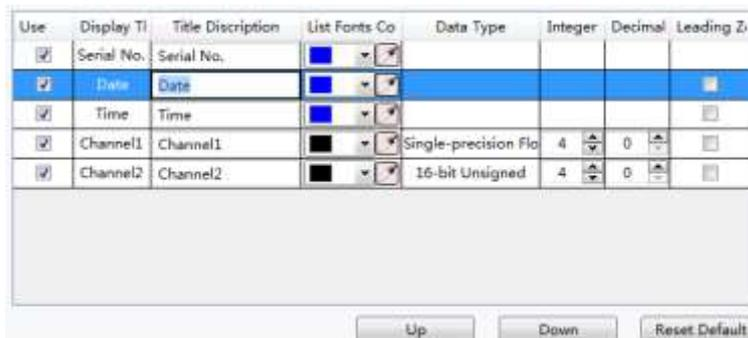
You can select the required contents to display in the title bar by checking in the "Use" column. For the order of the contents arrangement, you can use the button "Move Up" or "Move Down" to modify it. The content on the top row will display on the left of the Historical Data Display List. You can restore the default arrangement by clicking the button "Restore Default".
