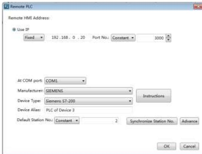
Click the button "OK" to confirm the settings and the "Remote PLC" device is added to the "Remote PLC" settings page.
