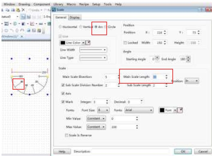
The start angle and the end angle can be set for the arc scale in the “Angle” property box. The settings and the effect are shown as below.
