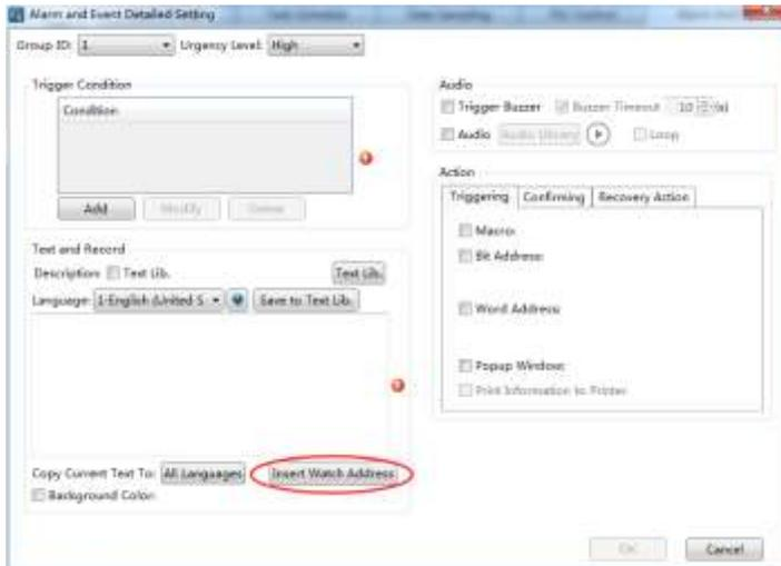
You can click the button as shown in the figure to enter the "Watch Address Table" ( path : Alarm and Event Display/Alarm and Events Login/Create/Insert Watch Address), you can also enter it through the tool bar(path: Library /Watch Address Table) .
