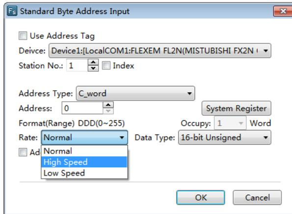
Certainly, you can use the address tag library. You need to prepare the data addresses in the address tag library before using them. Check the “Use Address Tag” in the “Standard Byte Address Tag” window and click the button “
