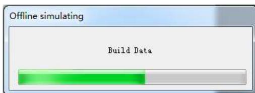
The project compiling needs a little time. There is a progress bar to indicate the compiling progress. The simulator window (Emulator) will open automatically after the compiling is finished.
