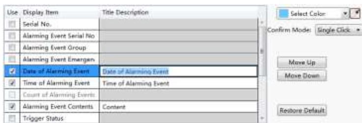
For the order of the contents arrangement, you can use the button "Move Up" or "Move Down" to modify it. The content on the top row will display on the left of the alarm list. You can restore the default arrangement by clicking the button "Restore Default".
