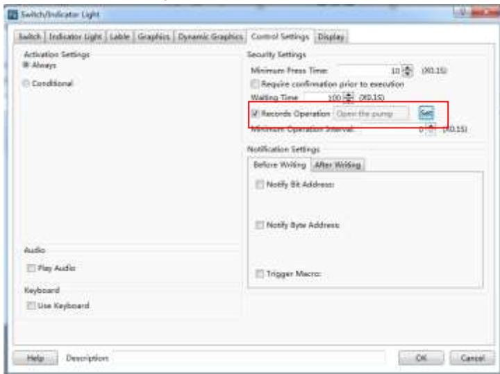
If you check this function, you can record the operations of the component and display the records in the operator Log. It is shown as below.
