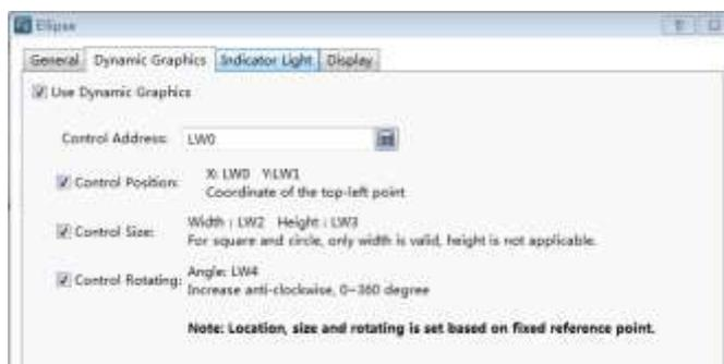
You can use the function of “Dynamic Graphics” if you want to adjust the position, the size and the rotation angle of the figure dynamically during running the HMI.
