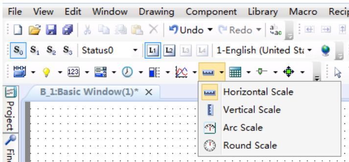
The “Horizontal Scale” is mainly used to display a progress bar. The “Vertical Scale” can be used to display the current liquid level of a tank or the charge state of a battery. The “Arc Scale” can display the value of a fuel meter, a speed meter, and other display devices. The “Round Scale” can display the revolution speed, the angle and other parameters.
