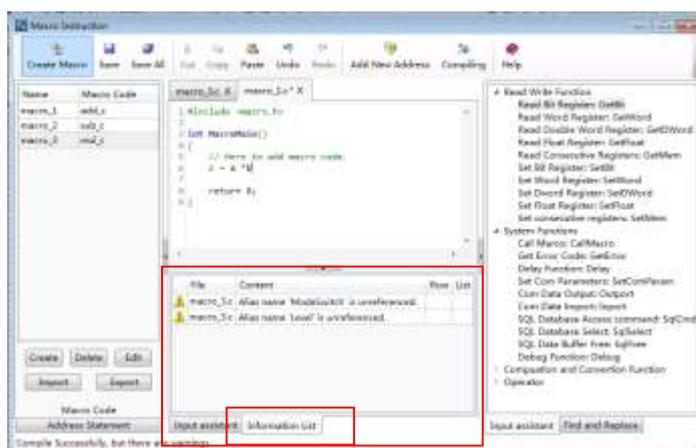
Information List window displays prompts and error messages when the macro compile. You can double-click the error message entry in the list if compiling errors occur. It will quickly navigate to the position where this error occurs.
