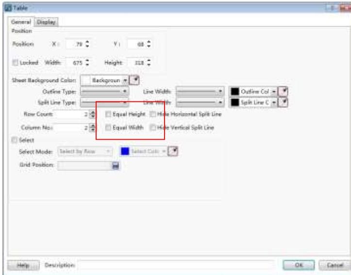
The difference with the “Fixed-width Table” is that the options “Equal Height” and “Equal Width” are not checked. Of course, you can check them and make the Fixed-height Table switch to the Fixed-width Table.
