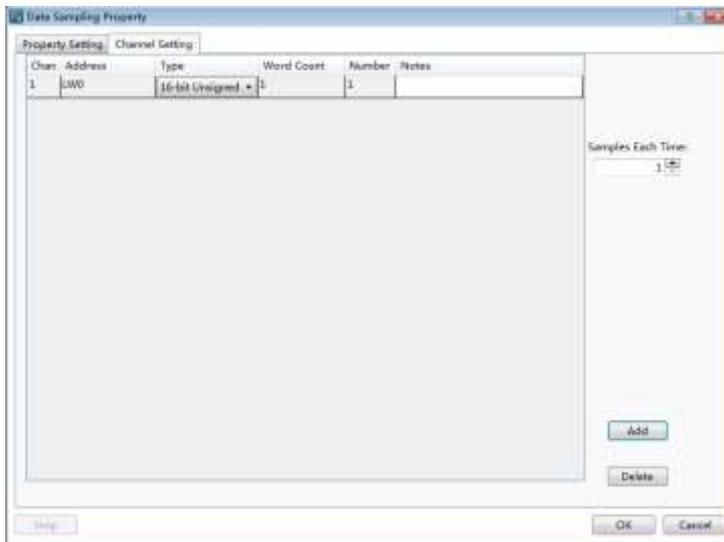
The "Address" refers to the start address of the data record. The "Type" of data record can be "16-bit Unsigned", "16-bit Signed", "32-bit Unsigned", "32-bit Signed", "16-bit BCD", "32-bit BCD", "Single-precision Floating-point Number" or "Character String". The maximum memory occupied is 64 word registers for the type of "Character String".
