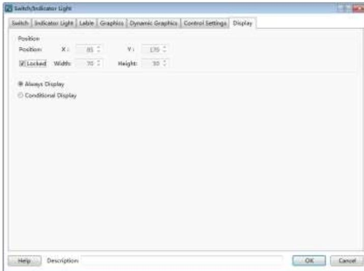
The position and size of the component cannot be changed if you check the “Locked” function. And there is a small lock icon on the component in the editing window. It is shown as below.
