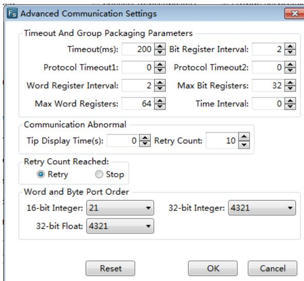
The parameters in the Advanced Communication Settings should not be modified. The optional modification may result in a communication failure or unexpected events occur. You can consult the factory technical staff to modify the advanced parameters based on your needs.
