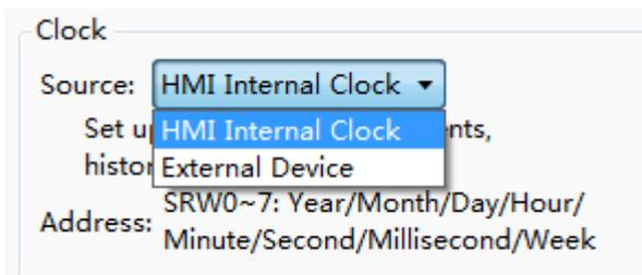
If you select the “HMI Internal Clock” as the HMI clock, SRW0~7 will be used to save the time source of events, historical data, etc.
