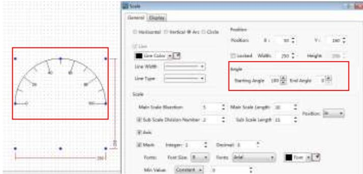
For the option “Position” in the “Scale” property box, the axis position of the scale can set “In”, “Out” and “Center”.
