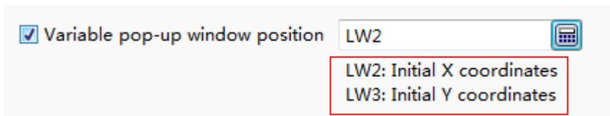
For the above example, check the option "Variable pop-up window position" and the first word register address of the window position control is set LW2. Then add two numeric value input components in your project for inputting the X and Y coordinates of the pop-up window. They are connected with LW2 and LW3 separately.
