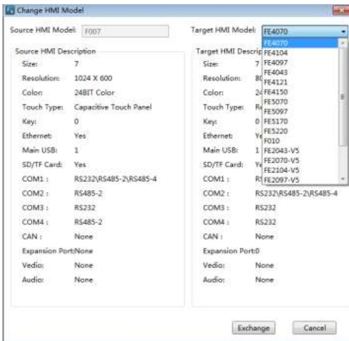
After you select the “Target HMI Model” for your project and click the button “Exchange” to confirm the setting, the project will be converted to adapt the new HMI device.
