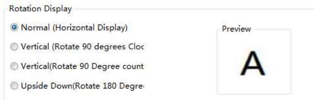
There are 4 rotation display effect. They are “Normal (Horizontal Display)”, Vertical (Rotate 90 degrees Clockwise), “Vertical (counterclockwise)” and “Upside down (Rotate 180 degrees)”. You can preview the display effect of the character “A” on the right area.
