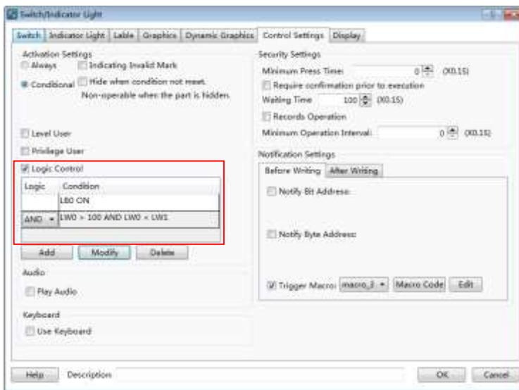
There is a relationship option in front of the second condition in the Logic Control list. The option can be set "AND" or "OR". It means the logic relationship between the previous User condition and the following condition. The component can be operated or display only if the result of all the conditions logic operation is true.
