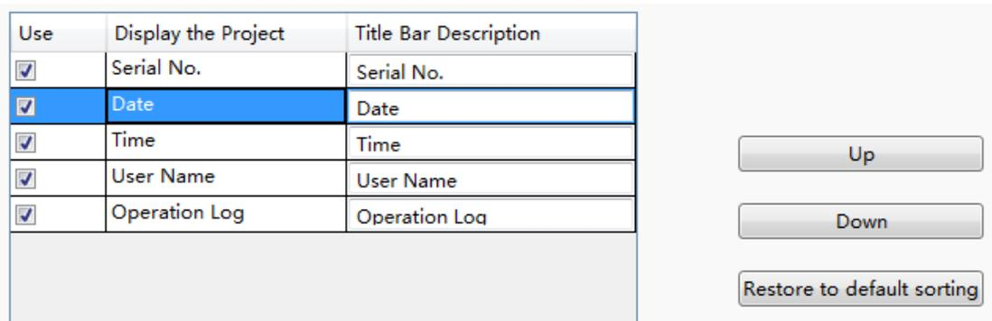
You can select the required contents to display in the title bar by checking in the “Use” column. For the order of the contents arrangement, you can use the button “Up” or “Down” to modify it. The content on the top row will display on the left of the Operator Log List. You can restore the default arrangement by clicking the button “Restore to default sorting”.
