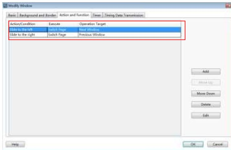
If you click the “Use Swiping Around” option, then the function of horizontal sliding will take effect, the function is only valid for the capacitive HMI.
