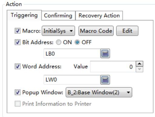
The actions of “Triggering” refers to the actions that they will be executed when the alarm or event occurs. The actions of “Confirming” refers to the actions that they will be executed when the alarm or event is acknowledged by manual. The actions of “Recovery Action” refers to the actions that they will be executed when the alarm or event exists.
