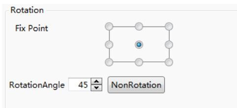
The function of “Rotation” can adjust the display angle of the components such as static graphics, vector graphics and other components. This function is a static function. That is, the display angel is not adjusted in the HMI if you set the display angle in the “Rotation” property. If you want to dynamically adjust the display angle of the graphics, please refer to: [Detailed manual/General functions/Dynamic Graphics](#).
