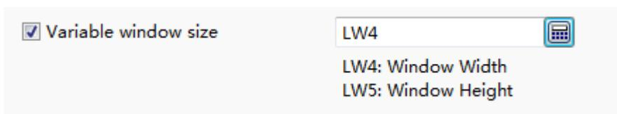
For the above example, check the option "Variable window size" and the first word register address of the window size control is set LW4. Then add two numeric value input components in your project for inputting the width and height of the pop-up window. They are connected with LW4 and LW5 separately.
