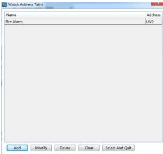
**Add:** You can add new watch address entry. Click "Add", set the watch address name, such as "Fire Alarm", and set the address of the watch entry, such as "local
