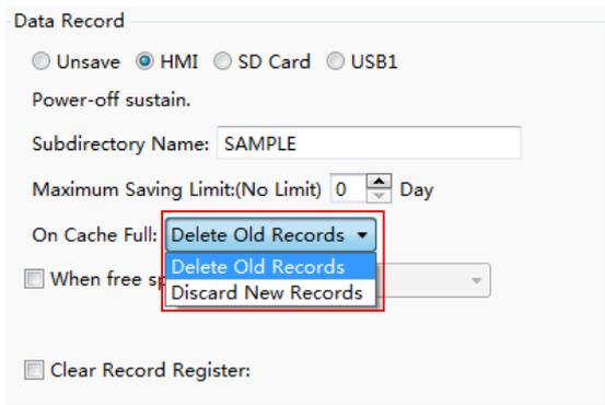
If you check the option “When frees pace is less than”, the action of “Notify Register” will be done when the free space is less than the specified capacity. The capacity range is 16KB ~ 2MB. You can set a bit register to notify. The bit register will be ON when the free Flash capacity is less than the specified.
