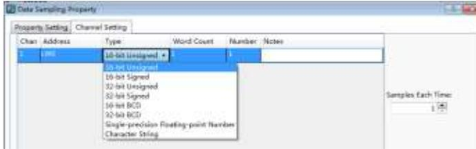
You can create many channels by clicking the button "Add". The addresses of the data record are continuous and specified automatically. It is shown as below.
