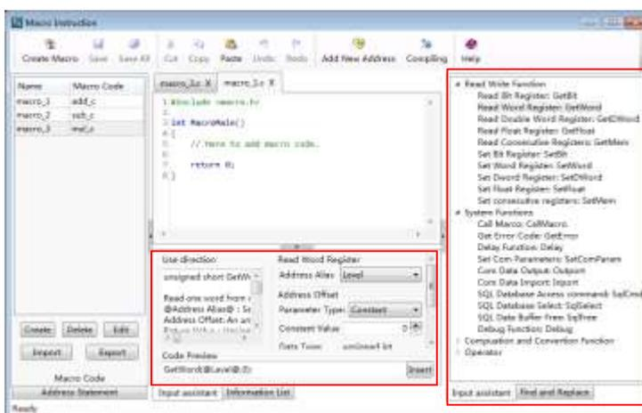
Input assistant Window on the right of the macro editor lists the built-in functions. It will display a detailed description of the function in the Input assistant Window at the lower middle position of the macro editor when you select a built-in function on the right window.
