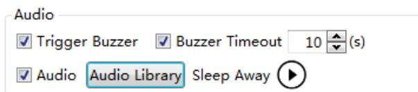
If the option “Trigger Buzzer” is checked, the internal buzzer of HMI will beep when an alarm occurs. If the option “Buzzer Timeout” is checked, you can set the beeping time of the buzzer. If the option “Audio” is checked, you can select an audio from the Audio Library as the sound of the alarm or event.
