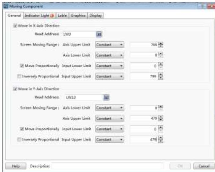
The option “Move in X-Axis Direction” refers to moving along the horizontal direction. The option “Move in Y-Axis Direction” refers to moving along the vertical direction. These two options can be checked together. That means moving in an oblique line direction. The angle of the oblique line can be computed based on the moving distance along the x-axis and along the y-axis.
