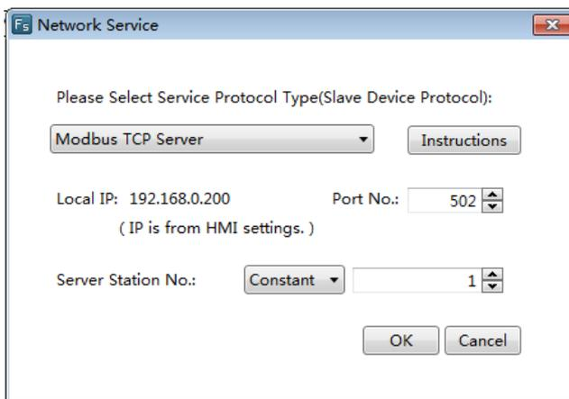
The Service Protocol Type supports Modbus TCP Server. It is referred to: Ethernet Service
