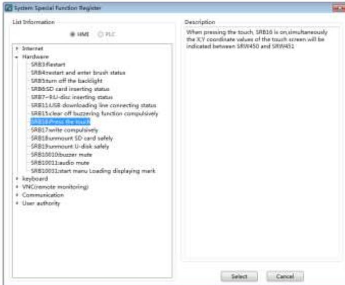
**Note:** "Word Register" and "Bit register" in HMI are two different areas, so the address does not overlap. For example, LW0 and LB0 are two registers that they are not related. SRW0 and SRB0 are also two different special system registers. But each word register can be divided into 16bit registers. For example, LW0 can be divided into 16bit registers: LW0.0 ~ 0.15.
