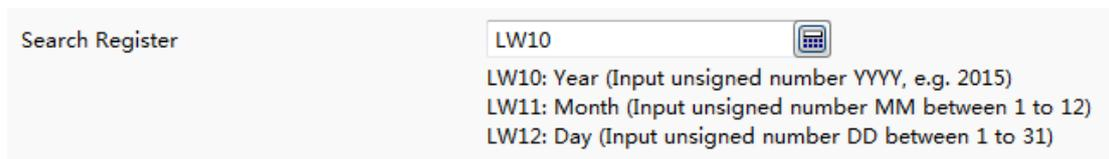
The screenshot shows the "Search Register" configuration. It features a label "Search Register" on the left and a text input field containing "LW10" with a calendar icon on the right. Below the input field, there is a legend: "LW10: Year (Input unsigned number YYYY, e.g. 2015)", "LW11: Month (Input unsigned number MM between 1 to 12)", and "LW12: Day (Input unsigned number DD between 1 to 31)".
